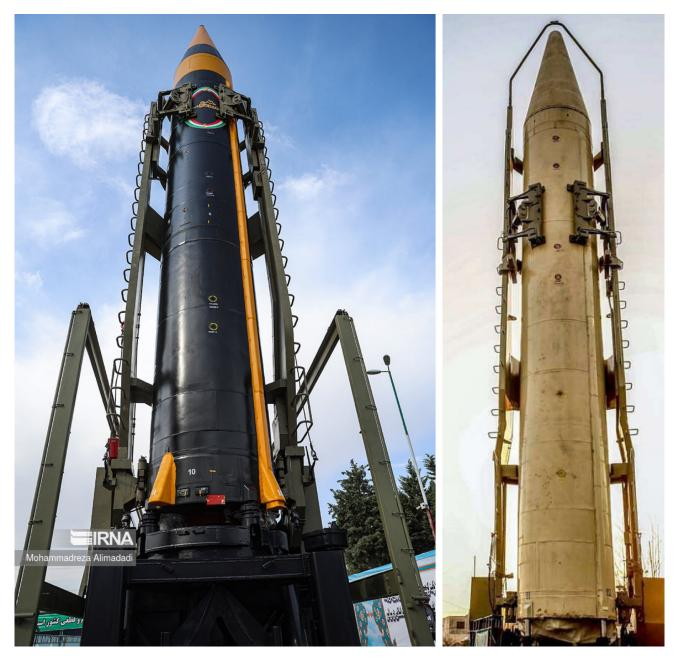
A side-by-side comparison of the Khoramshahr-1 (right) and 4 engineering prototypes shows modifications in areas like erector arms, nose cone, reentry vehicle skirt area, fuel- and oxidizer-tank configuration, missile-launchpad attachment points, and what appear to be added stabilizing fairings.
