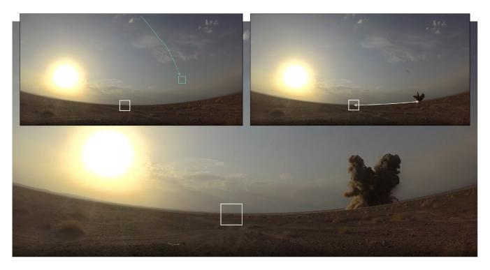
Iran claims pinpoint accuracy for its Khoramshahr-4 ballistic missile, but an examination of field test videos reveals the warhead impact to be off its apparent intended aimpoint. Stills of the warhead impact (green box, top left) show it missing its intended aimpoint (white boxes) by about a couple hundred meters.
