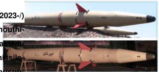
A supposed Haatem precision-guided ballistic missile at a September 2023 Houthi military parade (top) compared to an Iranian Kheibar Shekan ballistic missile (bottom). Close examination of the photo and video footage from the parade reveals that the Houthi example is a mockup lacking all the features of an operational missile (e.g., warhead-body attachment points, rivets, external connection ports). Photo credit: Al Masirah Television (top), IRIB-TV (bottom)
