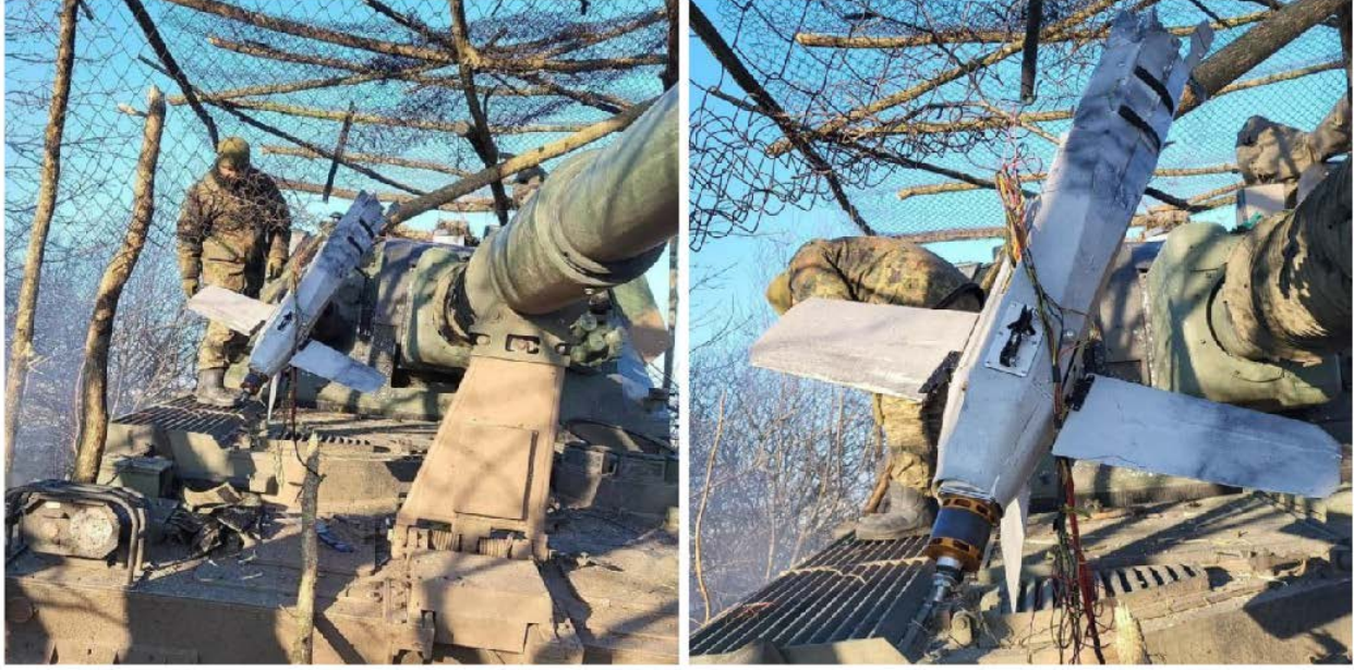
In Ukraine, debris from a Russian Lancet kamikaze drone that exploded prematurely after failing to penetrate protective chain-link fencing around a Ukrainian AHS Krab self-propelled howitzer artillery gun, January 2023. Credit: Kriegsforscher
