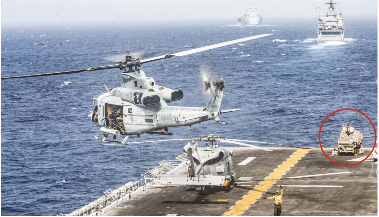
The I-MADIS system (circled) was used to down an Iranian drone while parked on the bow of the USS Boxer (LHD-4) as the ship transited the Strait of Hormuz, July 18, 2019. Credit: U.S. Marine Corps
