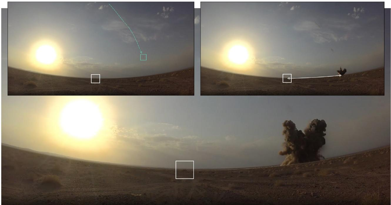
*Iran claims pinpoint accuracy for its Khoramshahr-4 ballistic missile, but an examination of field test videos reveals the warhead impact to be off its apparent intended aimpoint. Stills of the warhead impact (green box, top left) show it missing its intended aimpoint (white boxes) by about a couple hundred meters.*
