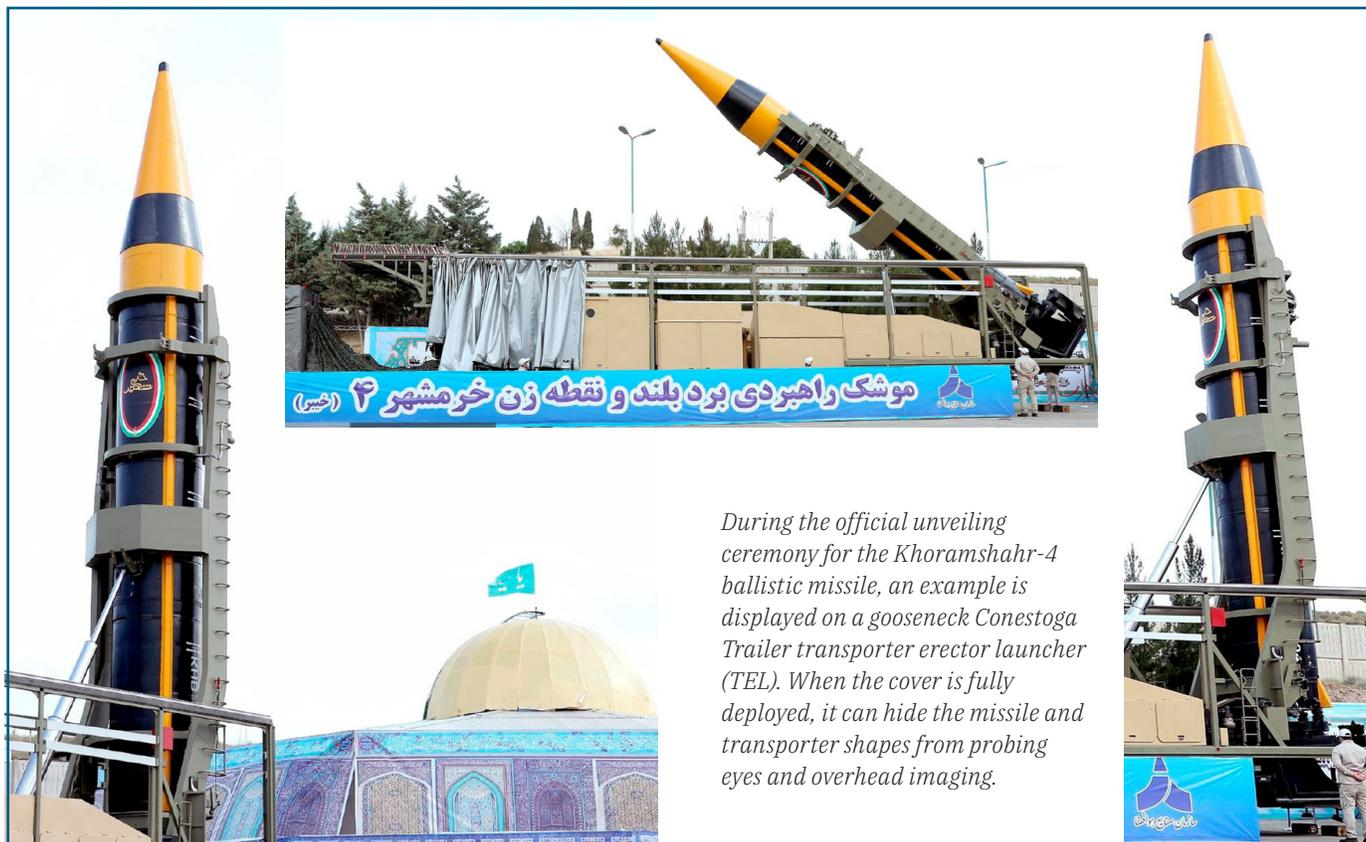
*During the official unveiling ceremony for the Khoramshahr-4 ballistic missile, an example is displayed on a gooseneck Conestoga Trailer transporter erector launcher (TEL). When the cover is fully deployed, it can hide the missile and transporter shapes from probing eyes and overhead imaging.*
