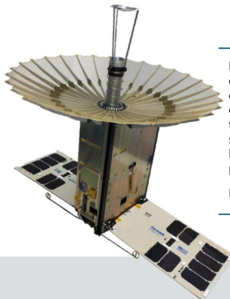
RainCube, a technology demonstrator 6U CubeSat experiment aimed at enabling precipitation radar technologies for earth science missions on a low-cost, quick-turnaround platform.
