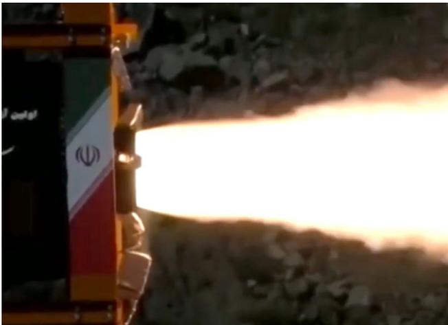
Two images of the Salman-1 rocket motor—about one meter in diameter—used for the second and possibly third stages of the Qased launch.
